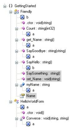
• Notice the currently highlighted **SaySomething** and **set\_Name** methods, as well as the **Name** property. Dotfuscator determined these items are not used in this application. As a result, Dotfuscator's Pruning feature is able to remove them, resulting in a more compact application.
